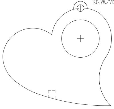
DRILL 13/8" DIAMETER HOLE OVERALL CLOCK SIZE: 17/16"
